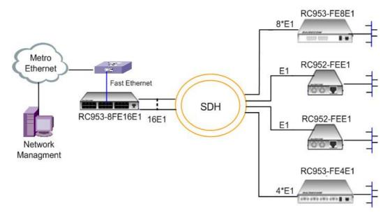
Figure 5-2 point-to-multi point topology
